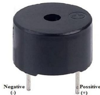
Fig 10. Buzzer Pin Configuration
